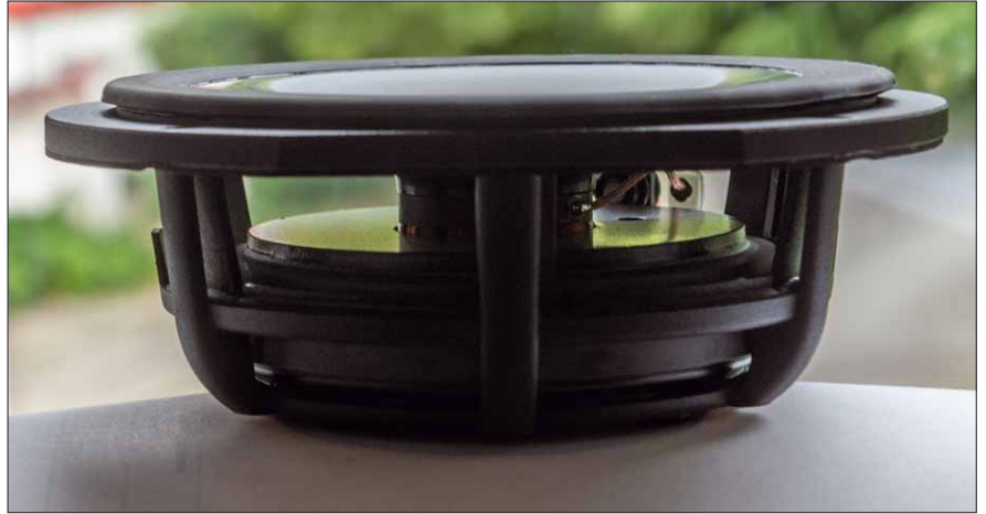
This is the brand new midrange driver without spider
