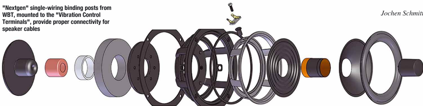
Die-cast aluminum on the outside, "technical plastic" on the inside: the dual-basket design of the midrange driver is one of Audio Physic's tried-and-tested means to instantly suppress sound-impairing resonances
