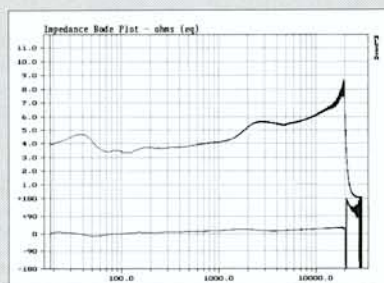
Fig.1 Audio Physic Caldera, electrical impedance (upper trace) and phase (lower) (1ohm/vertical div.).
